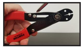
**2.** Squeeze the handles of the wire stripper to push the blades together; meanwhile, rotate the wire stripper while firmly holding the wire in place. Next, gently pull the wire stripper toward the shorter side of the wire to remove insulation.
