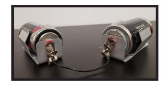
If you are using alligator clips, check that the metal clips are making full contact with the clips of the battery holder.
