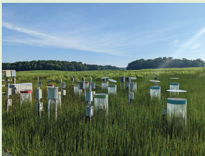
Figure 3.11: Automatic chambers setup in the Global Change Research Wetland at SERC.
